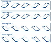
Before you install or remove the SIM card, use a pin to press the small cavity untill the SIM cassette pops out.
