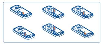
To release the microSD card holder, slide it in the direction of the arrow and lift it. Then insert the microSD card with the golden contact downward. Finally, turn down the microSD holder and slide it in the opposite direction to lock it.
