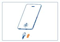
Connect battery charger to your phone and plug into the socket. If the battery is very low, there will be no indication that power is being received until the charge is sufficient to show the charging status bar. To reduce power consumption and energy waste, once the battery is fully charged, disconnect your charger from the plug; switch off Wi-Fi, GPS, Bluetooth or background-running apps when not in use; reduce the backlight time, etc.
