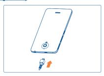
Connect battery charger to your phone and plug into the socket. If the battery is very low, there will be no indication that power is being received until the charge is sufficient to show the charging status bar. To reduce power consumption and energy waste, once the battery is fully charged, disconnect your charger from the plug; switch off Wi-Fi, GPS, Bluetooth or background-running apps when not in use; reduce the backlight time, etc.
